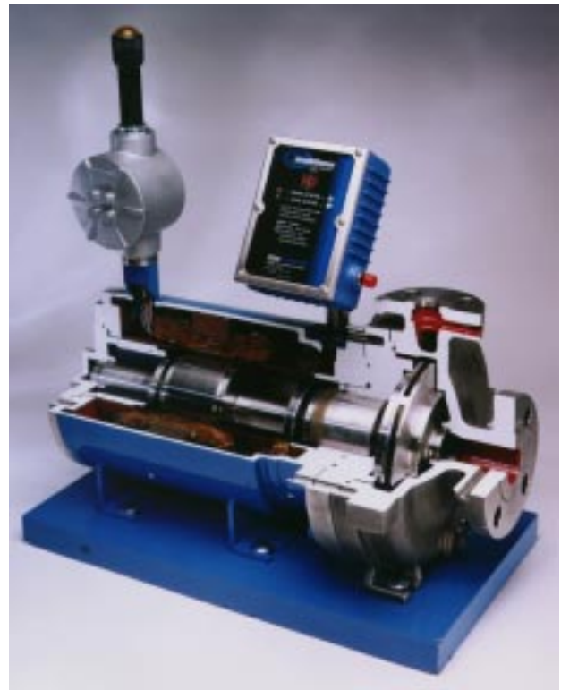
Chempump NC Series Cut-Away
